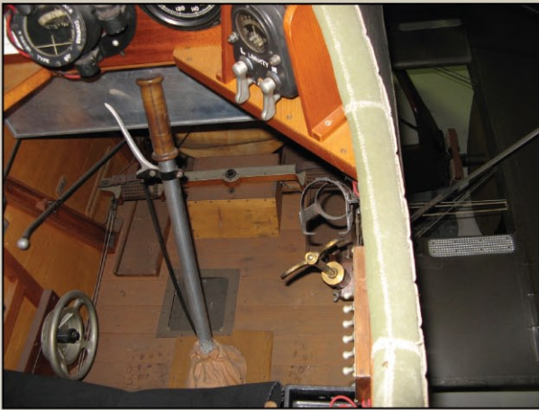
Control column (A22) with firing handle for the Vickers. Note the bomb sighting hole in the floor.
