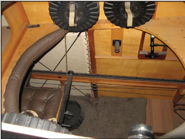
Observer's throttle (A29), seat and Lewis gun ammunition drums (R21). Note the interior colour of the linen fuselage covering.
