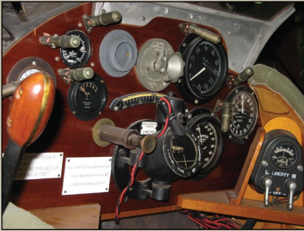
Instrument board detail from F1010 after full restoration to WW1 specifications. Note that post war instrument panels were noticeably different.
