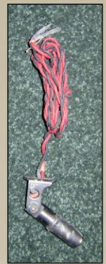
Instrument board lamp and electrical wire.
