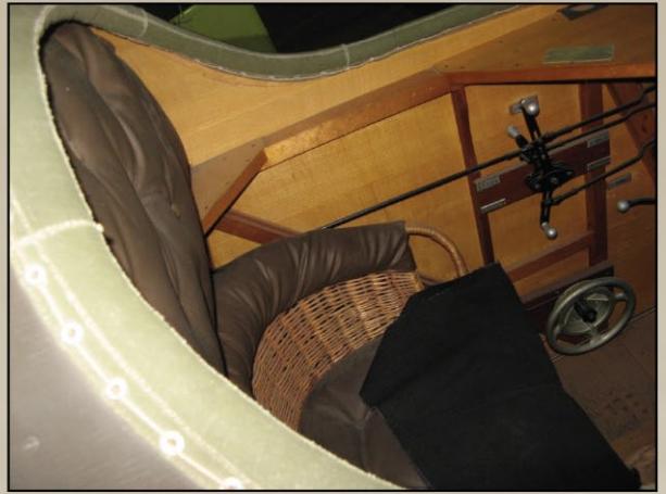
Pilot's seat, throttle (A8) and tailplane elevating gear (A4) details.
