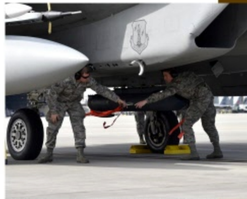
During their deployment, the Bats routinely carried the LM Sniper XR Pod on their centerline station
