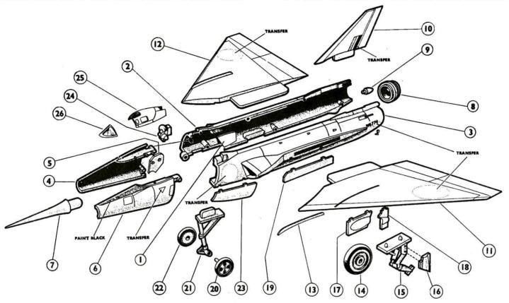
Incorporated in this model is a working "Droop Snoot" nose, as in the real aircraft. The nose of the fuselage is designed to drop to an angle of  $10^\circ$  to give the pilot a better view when approaching to land at the steep angle of attack that this type of aircraft has to maintain.
