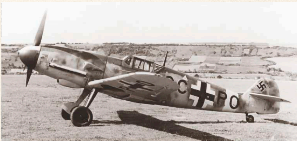
Bf 109 G-2 WNr. 14246. The aircraft has the smaller landing gear wheels (650x150 mm), with retractable smaller tail wheel (290x110 mm) and without bulges above the undercarriage wheel well on the upper surface of the wing.
