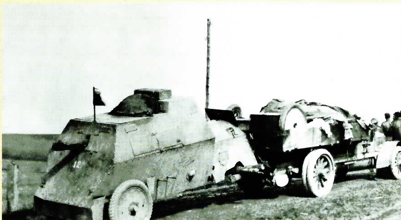
Illustration 4. 3-ton Saurer truck evacuates a damaged Russo-Balt armored car ahead of the cannon-armed Mannesmann-Mulag armored car. 1915.
