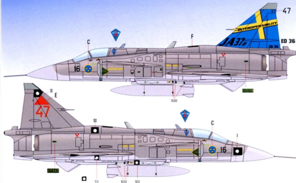
JA 37Di, 37347, 47- FC 2002. This airframe served as prototype for the Di modification. ED 36 indicates the Edit 36 software. The black/white dot-markings on the right side are test validation markings. The modification included capability to carry the Rb 99 AMRAMM Air to Air missiles. Later the F16 wing numbers were removed and a orange band applied around the nose (300 mm wide and black dashed in this view) indicated that the a/c was operated by the FC (Försökscentralen - The Test Establishment).
