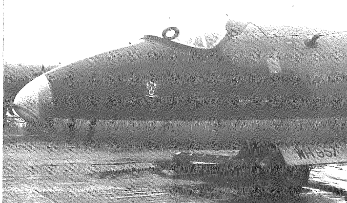
Port nose of WH957 showing the more recent application of the City of Derby coat of arms in lieu of the squadron badge, denoting the squadron's long association with this famous city. Again several of the stencil markings are visible, also the aerial mast on this side only.
