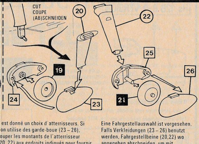
A choice of undercarriage is given. If spats (23-26) are used, cut undercarriage legs (20, 22) where indicated to provide locating lugs.
