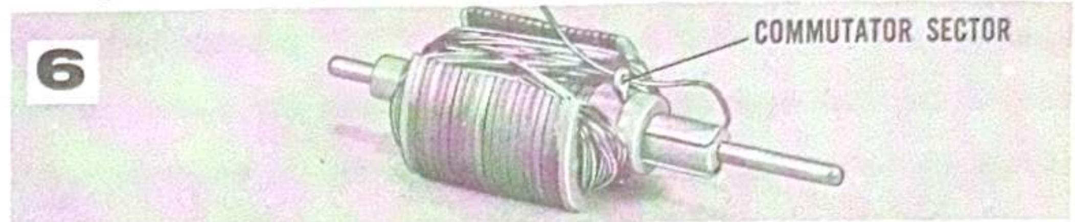
When winding is completed, take loose end of wire and clean  $\frac{3}{8}$ " of insulation off of wire as in Step No. 4. Now put end of wire through hole of second commutator sector and twist around sector as shown.
